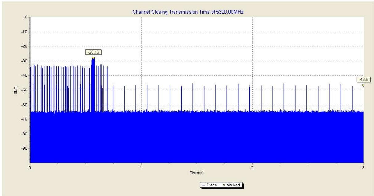
The closing transmission time is as the figure, and the result is 117ms
