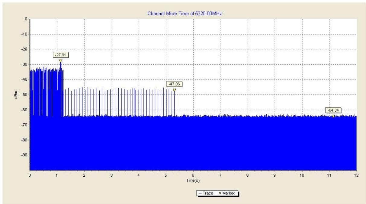
The channel move time is as the figure. It shows the time of the radar and the client pulses. The figure shows that the client stops transmission within 10 seconds, and no transmissions occur after 10 seconds later of the radar burst signal.
