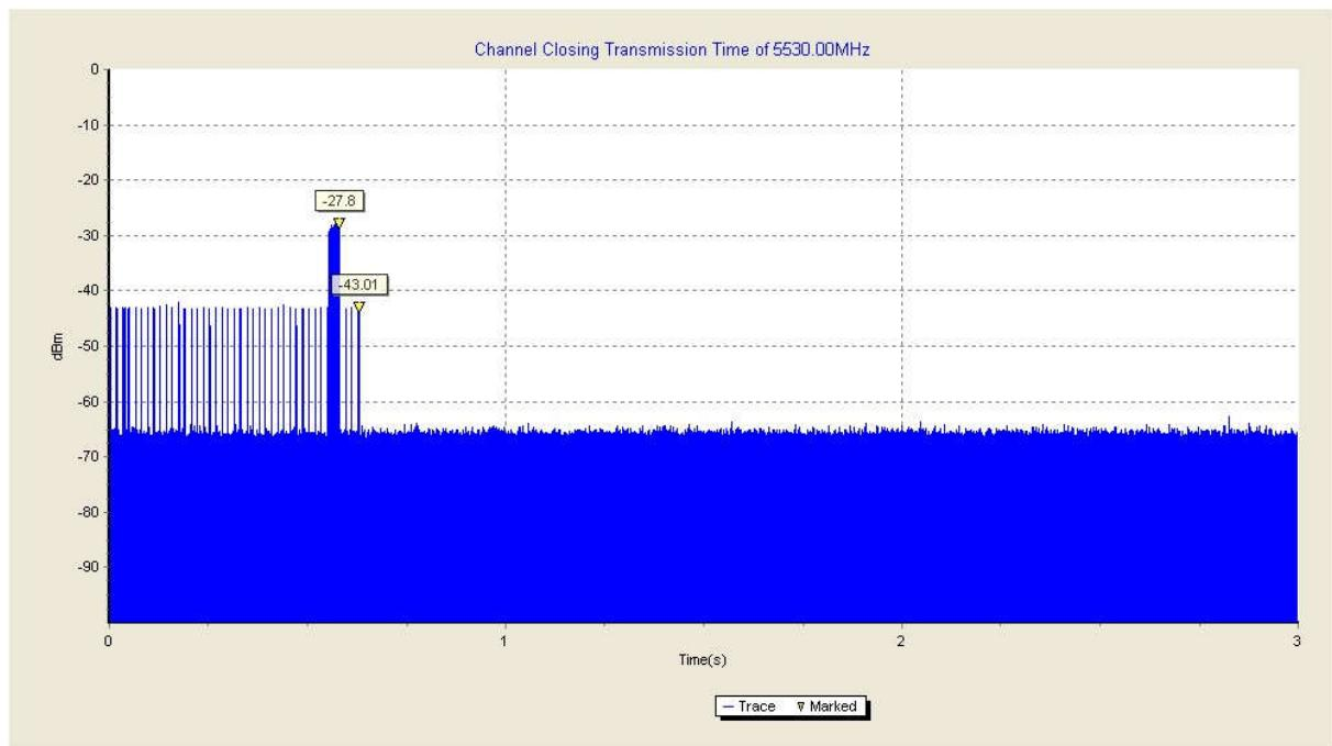
The closing transmission time is as the figure, and the result is 71ms
