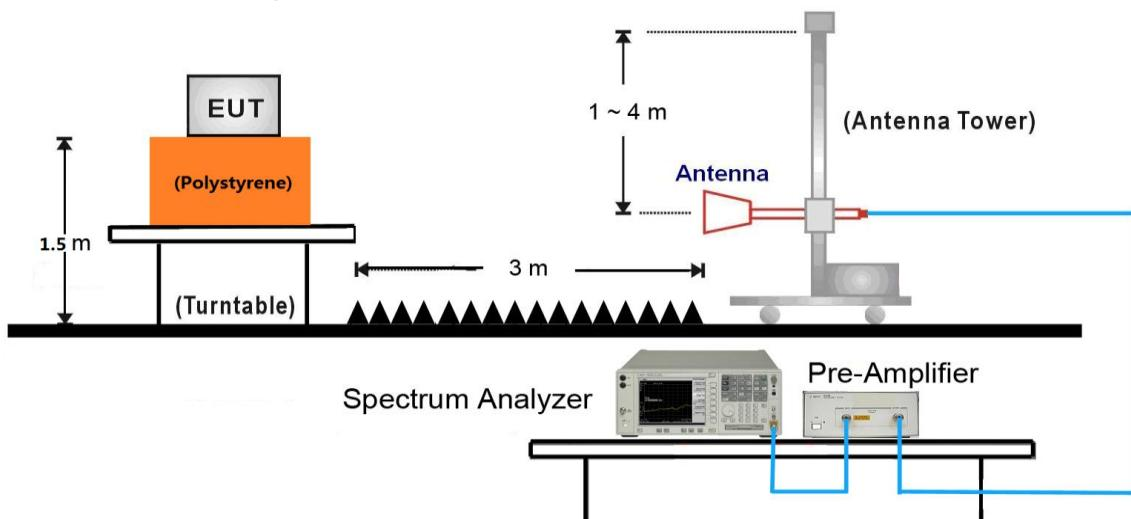
18GHz ~40GHz Test Setup:
