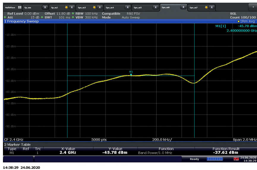
BT LE 2M Low Band Edge (Average Measurement). Limit is -32.18 dBm. Margin is -5.44 dB. (The highest level of the desired power within the band is -2.18 dBm)
