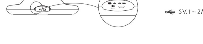
The power of speakers can be supplied by standard Tablet USB adaptor(DC 5.0V/1A-2A). Switch the Product to USB mode while supplying power through USB adaptors.
