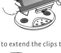
2. Push the button to extend the clips to maximum.
