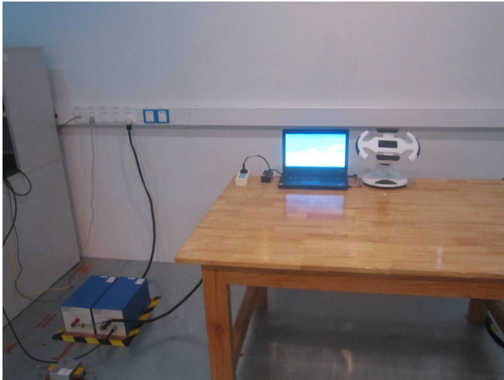
Conducted Emissions Test Setup Front View
