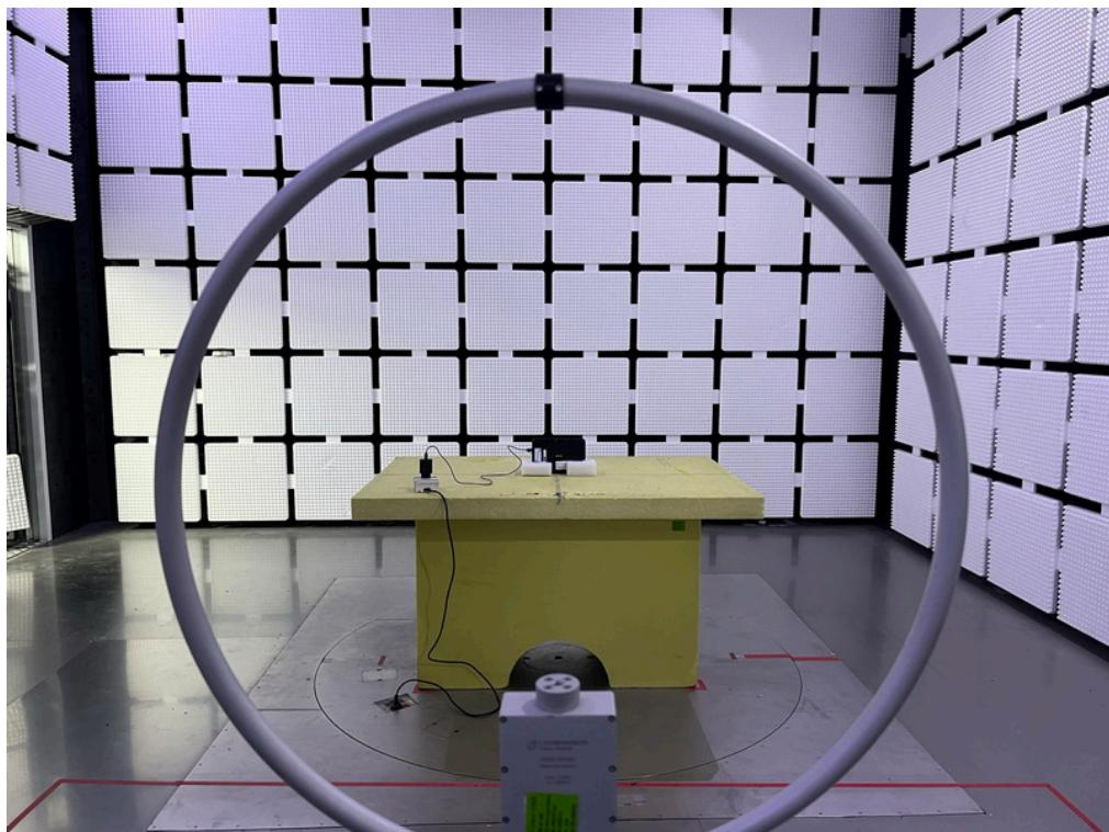
**Radiated Emissions Test Photos****30 MHz to 1000 MHz**
