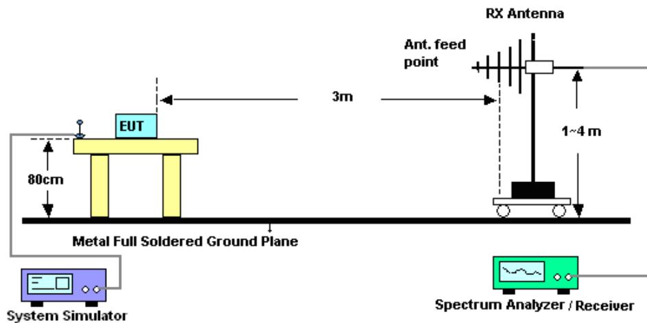
For radiated test above 1GHz
