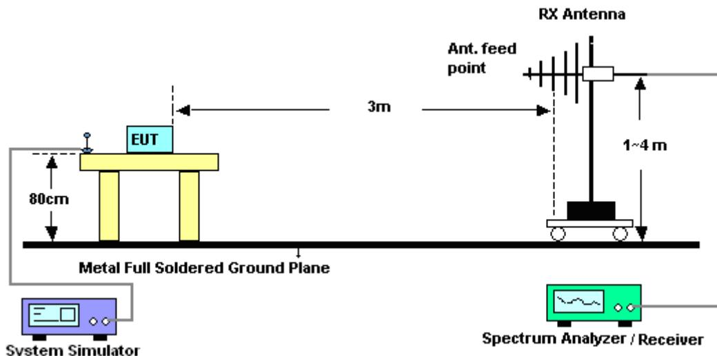
For radiated test above 1GHz
