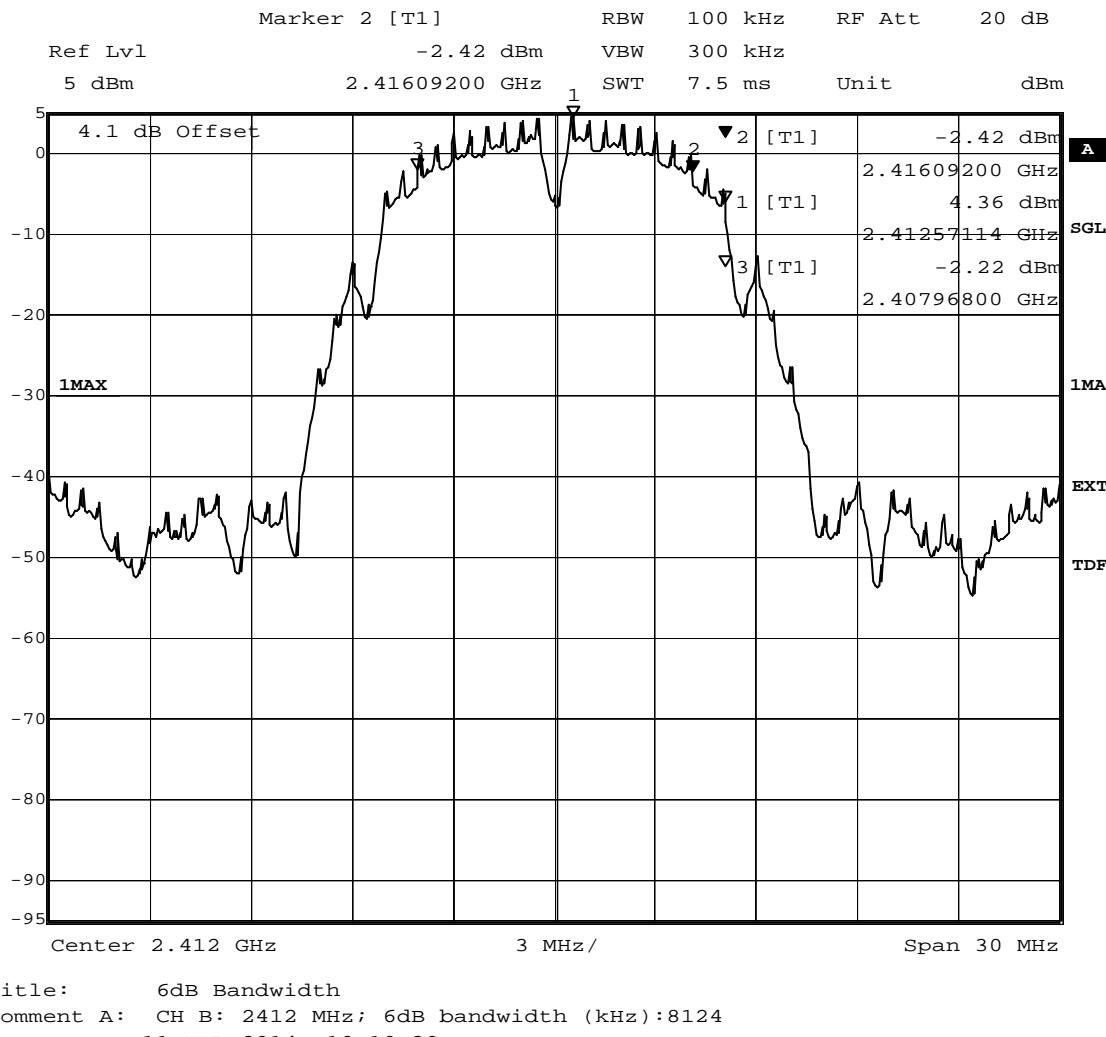
6 dB bandwidth at 2412 MHz, WLAN b-Mode; 20 MHz; 1 Mbit/s
