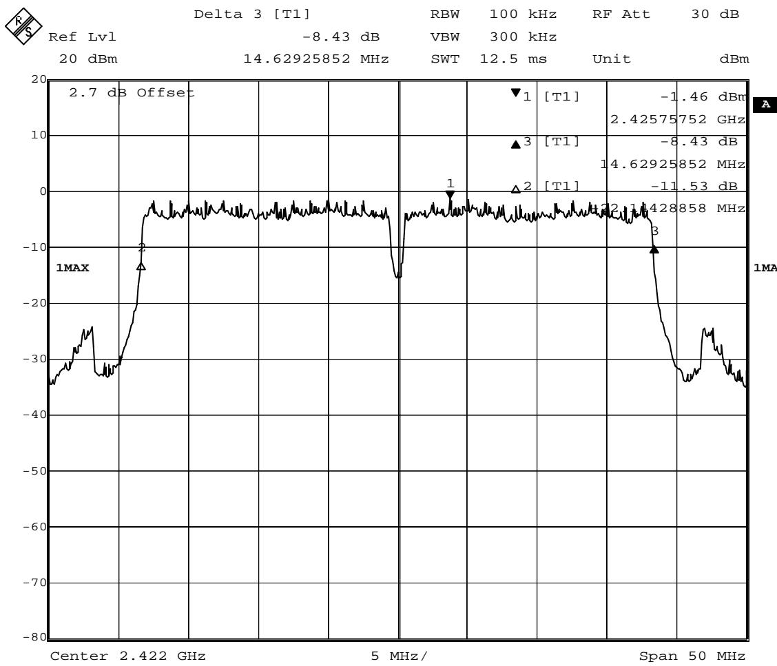
6 dB bandwidth at 2412 MHz, WLAN n-Mode; 40 MHz; 300 Mbit/s
