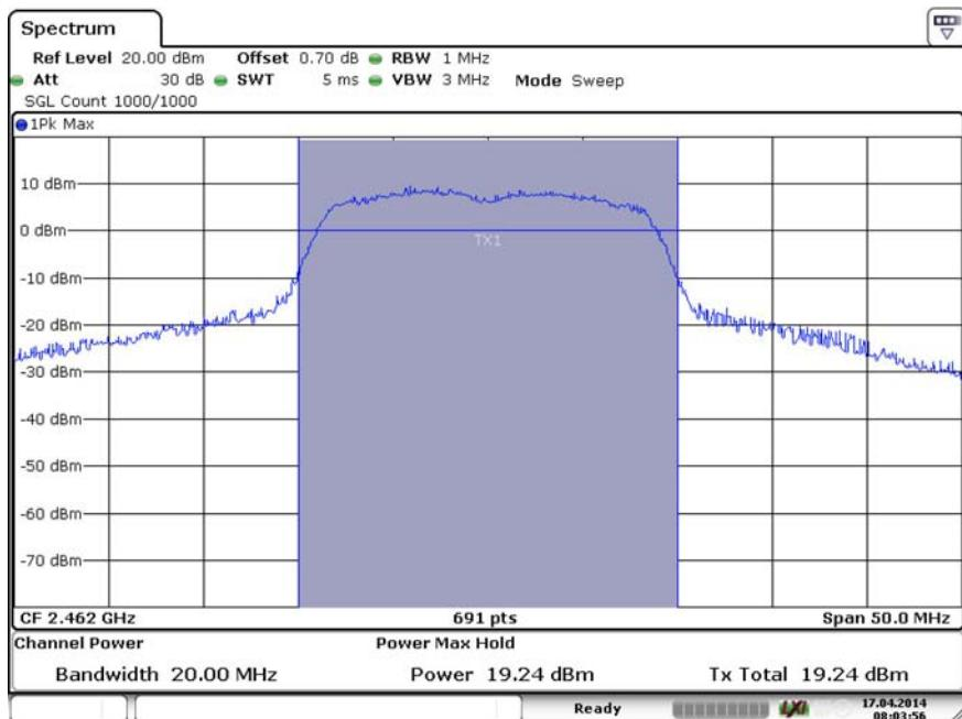
Peak output power, 2462 MHz, WLAN n-Mode; 20 MHz; 72.2 Mbit/s
