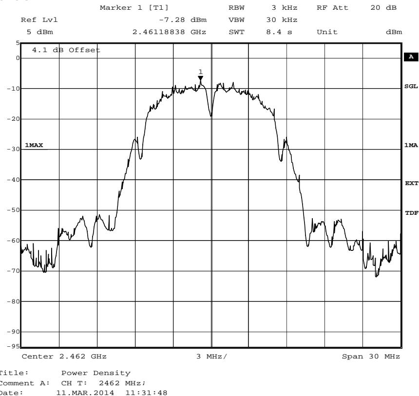
Remark: The plot contains the antenna gain
