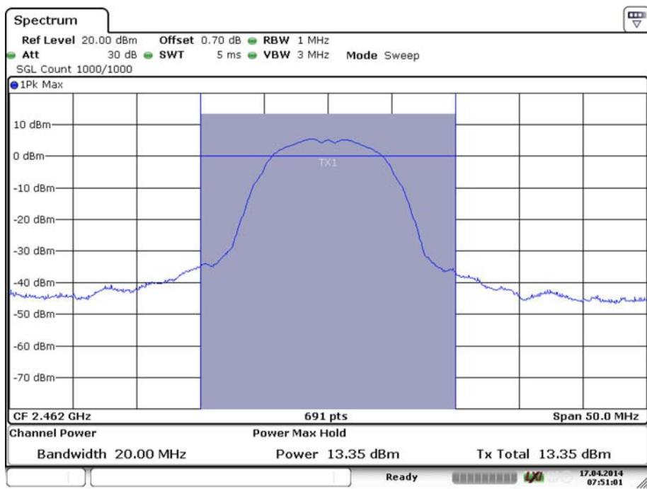
Peak output power, 2462 MHz, WLAN b-Mode; 20 MHz; 1 Mbit/s
