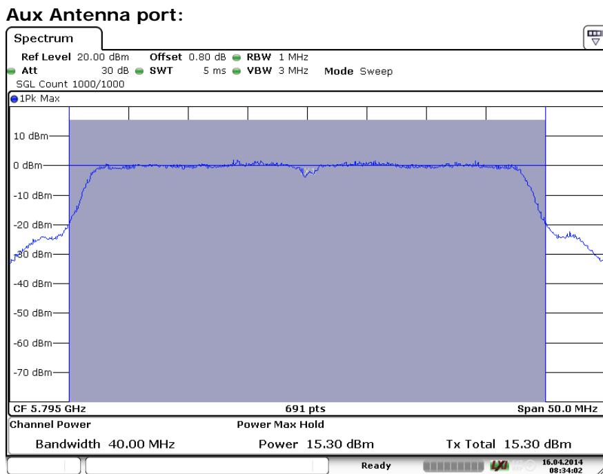
Peak output power, 5795 MHz, WLAN n-Mode; 40 MHz; 300 Mbit/s
