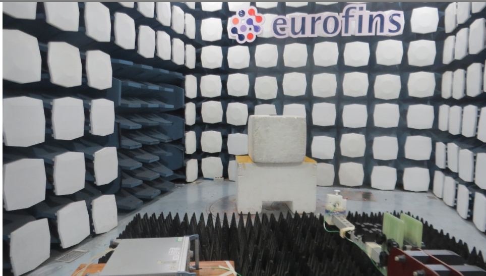
Picture 1 Radiated Emission Test Setup
