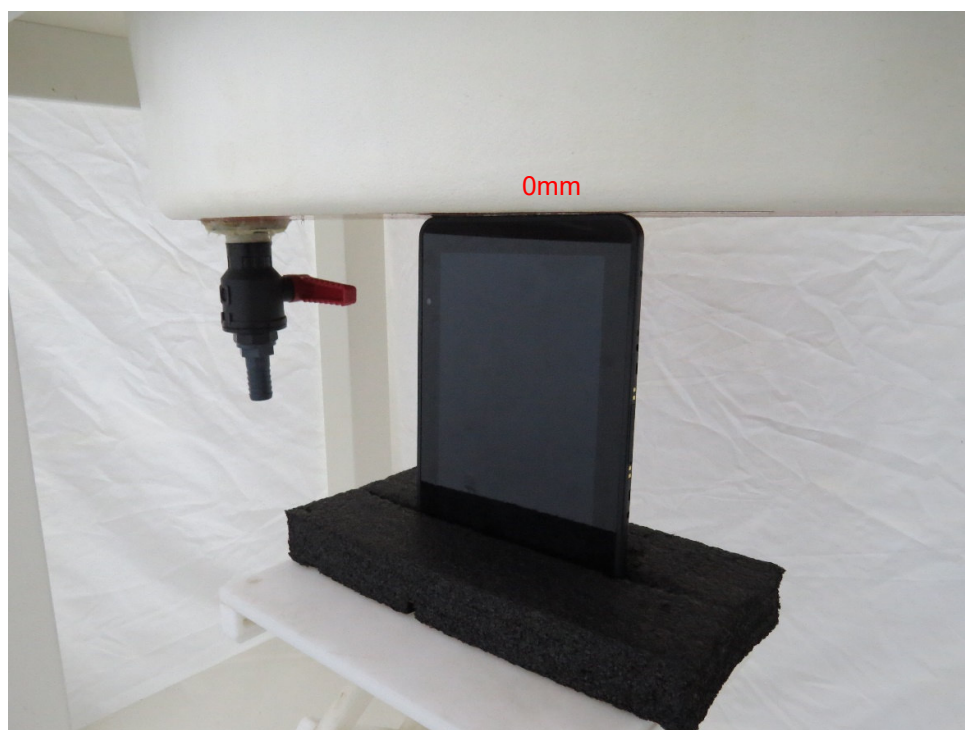
Picture 2: Right Side, the distance from EUT to the bottom of the Phantom is 0mm
