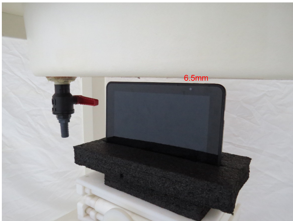
Picture 6: Top Side, the distance from EUT to the bottom of the Phantom is 6.5mm
