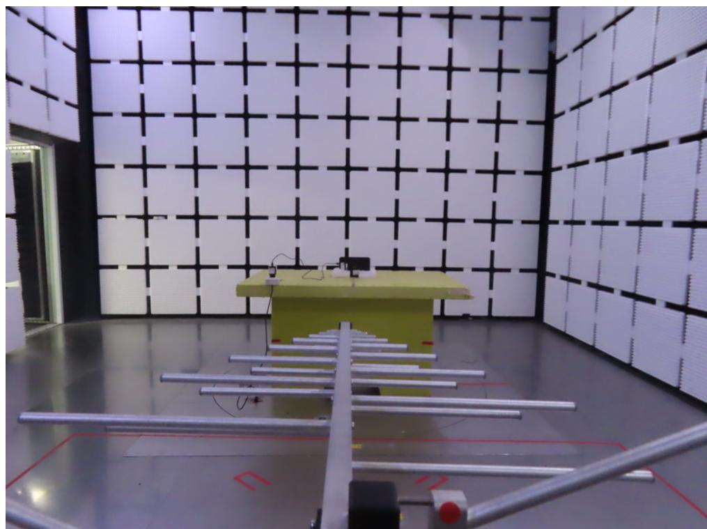
**Radiated Emissions Test Photos****Band edge & Harmonic(1 GHz to 18 GHz)**
