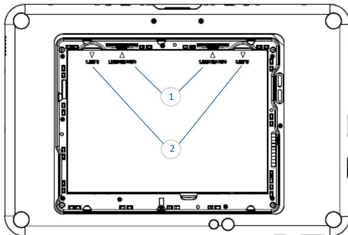
The memory card can be inserted on the upper side, please ensure you insert it in the right direction as shown on the picture.
