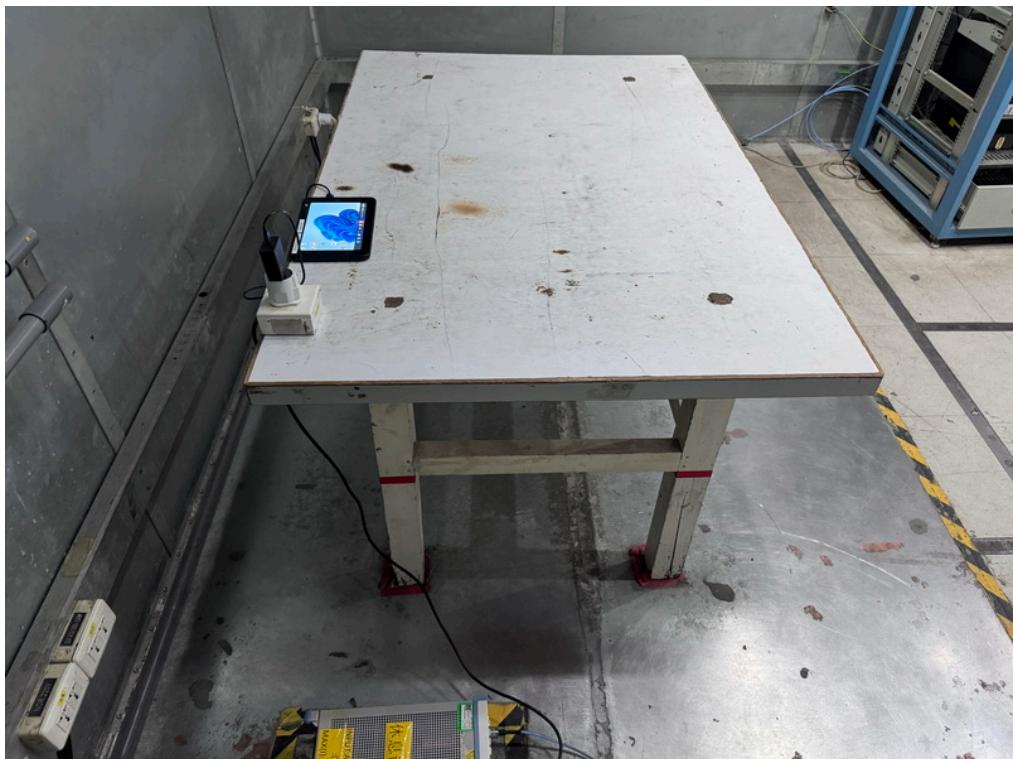
**Radiated Emissions Test Photos****9 kHz to 30 MHz**
