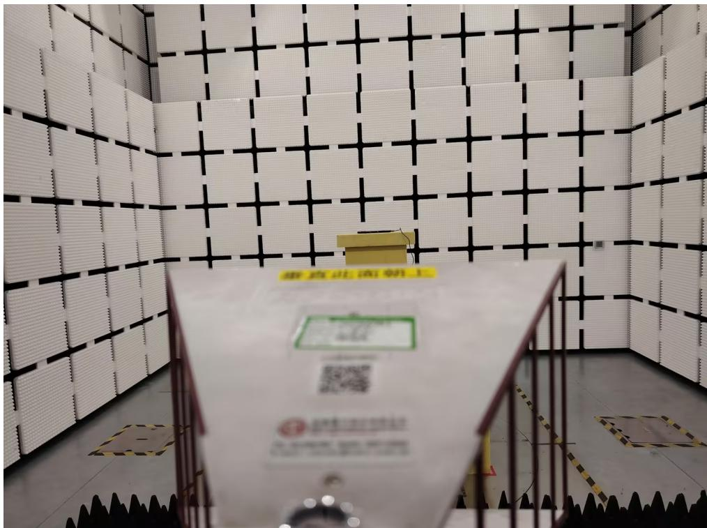
**Radiated Emissions Test Photos****Harmonic(18 GHz to 26.5 GHz)**
