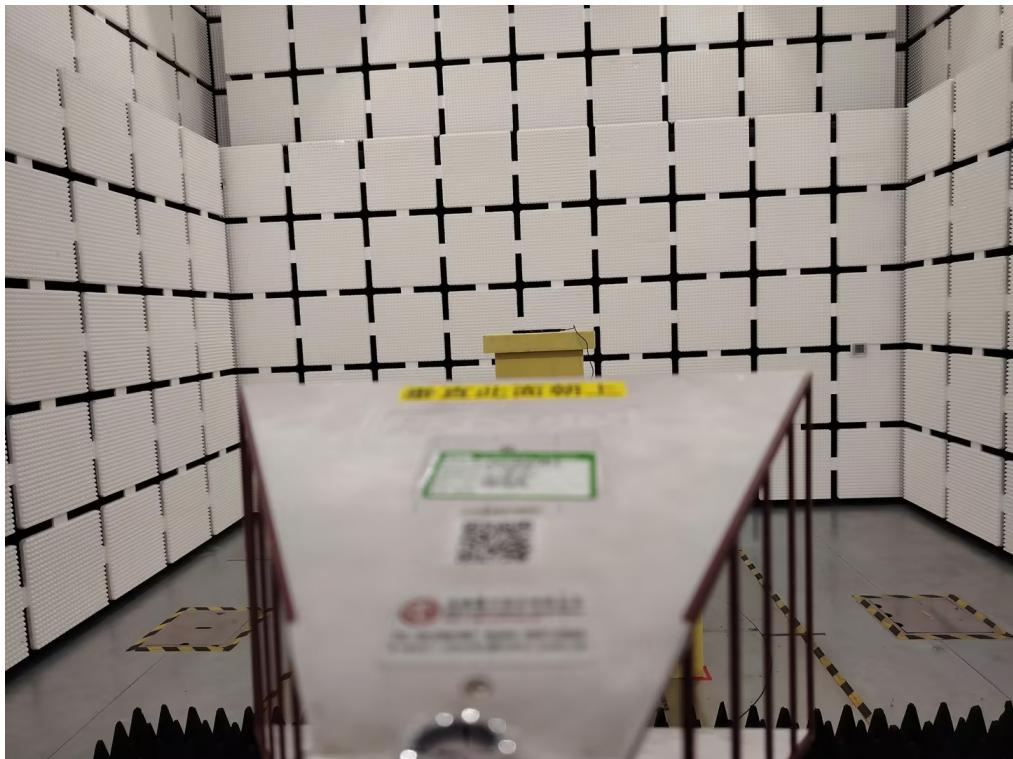
**Radiated Emissions Test Photos****Harmonic(18 GHz to 26.5 GHz)**
