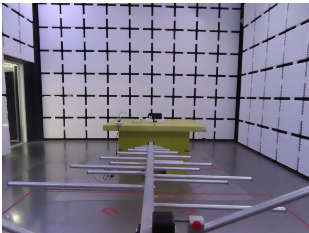
**Radiated Emissions Test Photos****Band edge & Harmonic(1 GHz to 18 GHz)**
