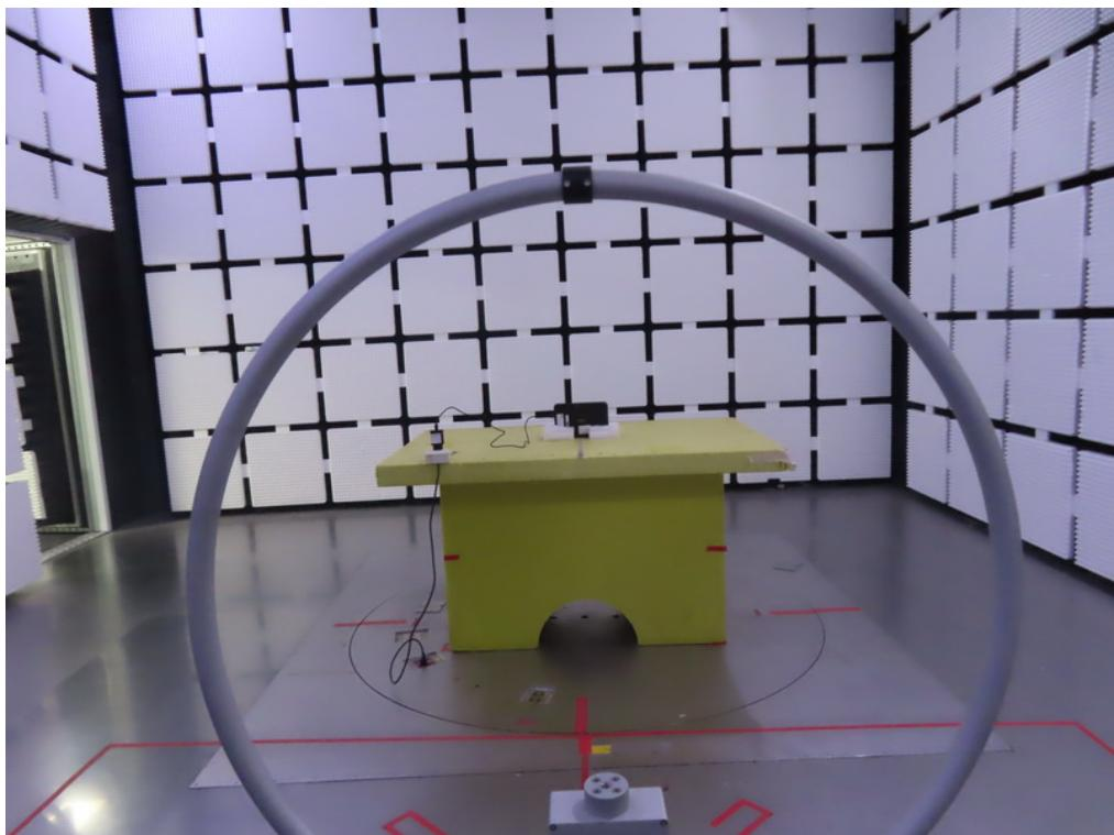
**Radiated Emissions Test Photos****30 MHz to 1000 MHz**
