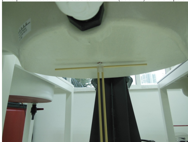
Photo of Dipole Setup
