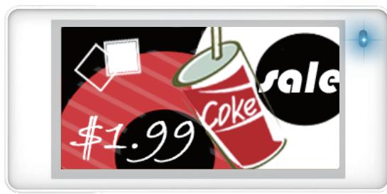
DS026 is a 2.6-inch super-thin ESL independently developed by MinewTag, utilizing the latest Bluetooth® Low Energy 5.0 Technology. It features a 7.8mm ultra-thin design, secure and fast data transfer, and agile, flexible screen refresh. Adopting the latest E-ink display technology, DS026 provides a fully-graphic display and paperlike appearance. With the 2.5D transparent shell, it delivers a nearly 180° viewing angle for excellent readability.
