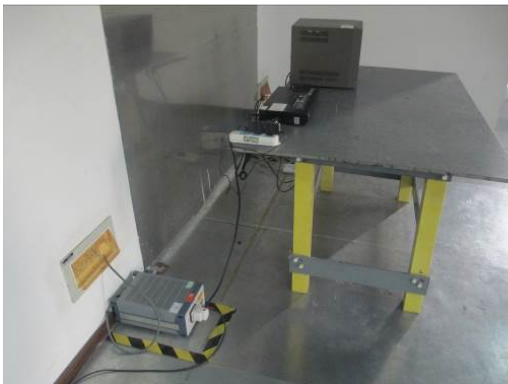
Conducted Emissions Test Setup Side View
