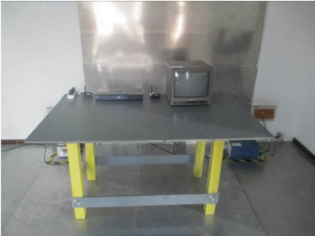
Conducted Emissions Test Setup Front View
