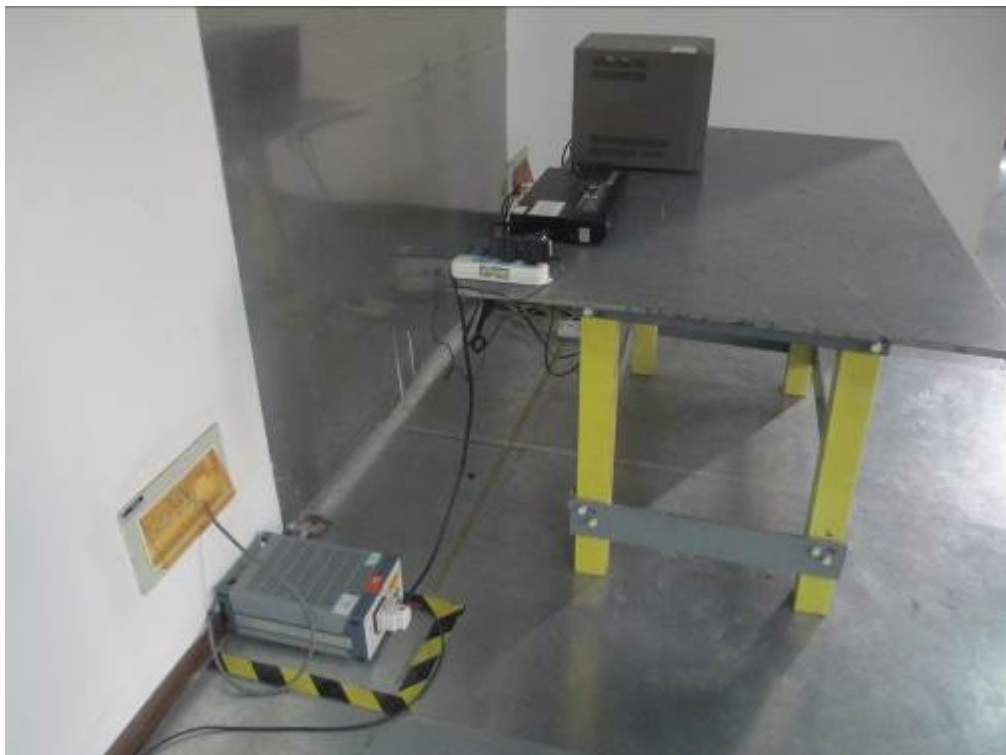
Conducted Emissions Test Setup Side View
