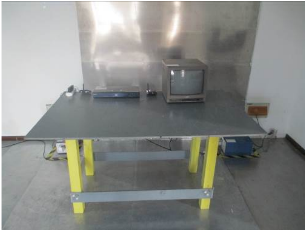
Conducted Emissions Test Setup Front View
