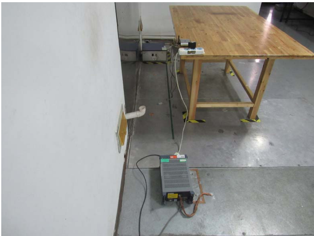
Conducted Emissions Setup Side View
