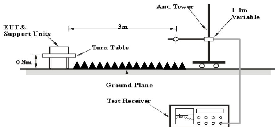
The radiated emission tests were performed at the 3 meters distance in chamber, using the setup accordance with the ANSI C63.4-2014. The specification used was the FCC Part 15.109 Class B limits.
