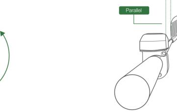
Attach shaft sensor just below the grip with charging contacts pointing down.
