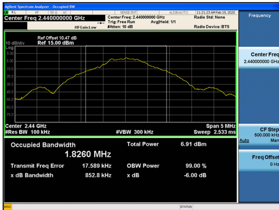
6 dB Bandwidth plot (Mid-CH 19)
