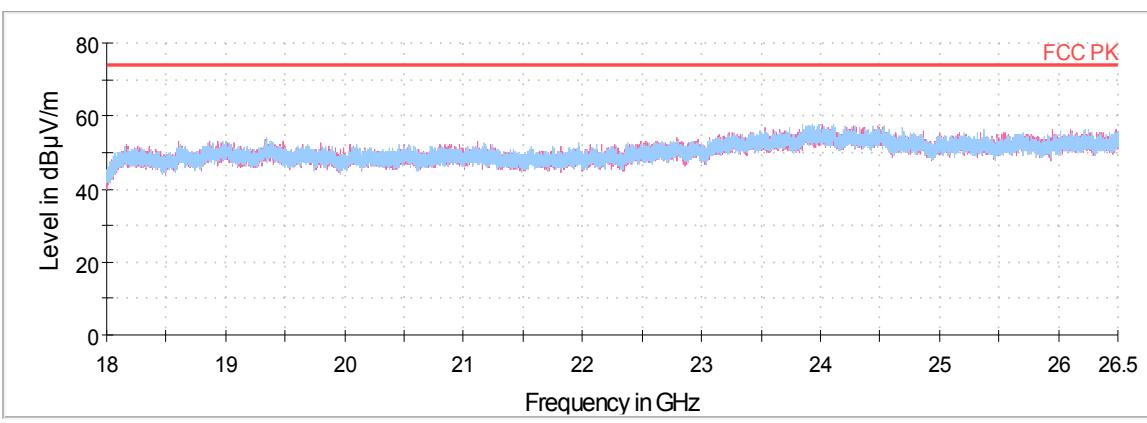
**Test results (Above 1 000 MHz) Worst case: 2MBits/s(255 Bytes)****Low Channel**
