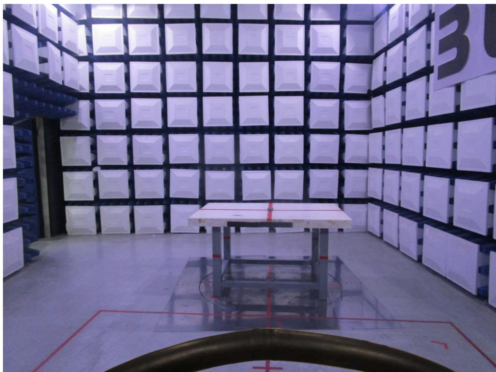
**Radiated Emissions Test Photos****30 MHz to 1000 MHz**
