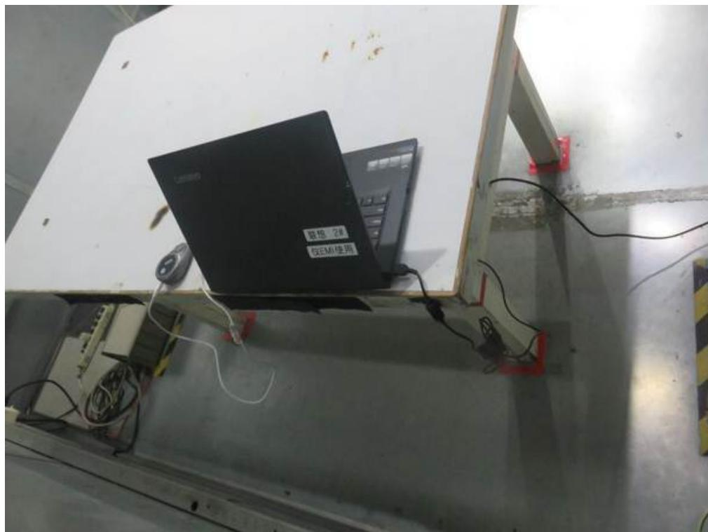
**Radiated Emissions Test Photos****9 kHz to 30 MHz**
