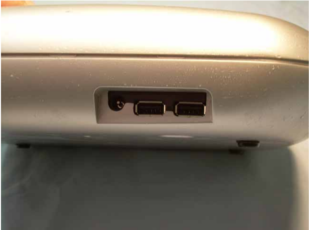
Photograph 7 – View of the Power and USB Ports of the EUT
