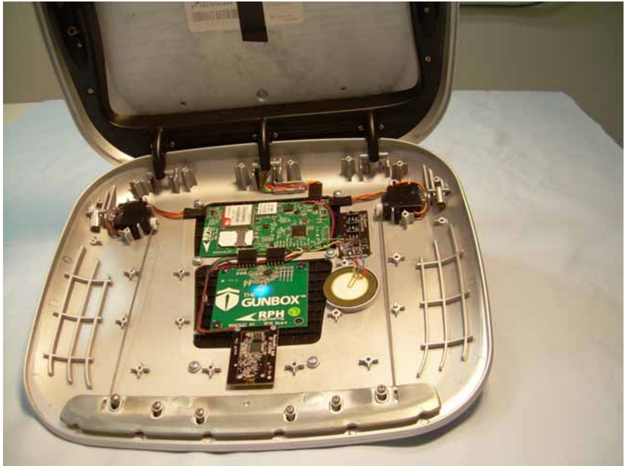
Photograph 9 – Location of the PCBs Except Power PCB
