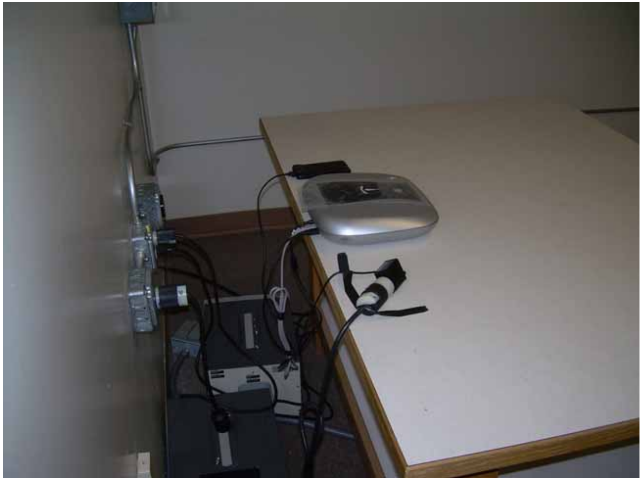
Photograph 4 – Back View Conducted Disturbance Worst Case Configuration
