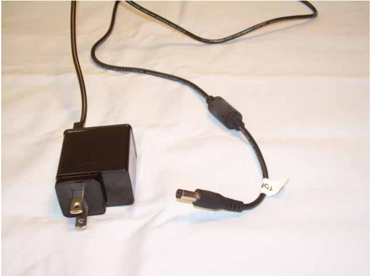
Photograph 11 – View of the Power Supply with Molded on Ferrite
