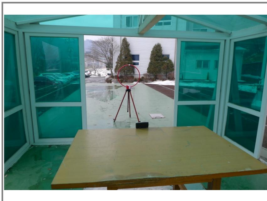
**Photo of radiated spurious emission at 30 MHz ~ 1 000 MHz**
