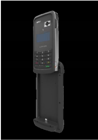
1) Put Brain in the line with the Sled rail.
