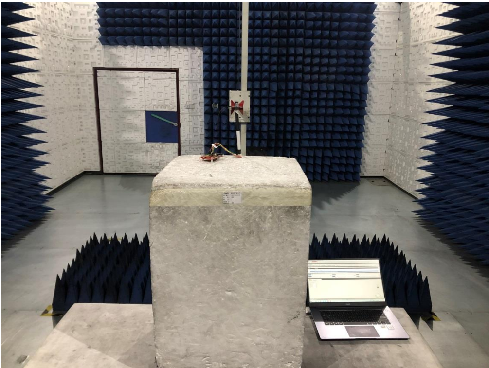
RADIATED EMISSION TEST SETUP ABOVE 1GHZ
