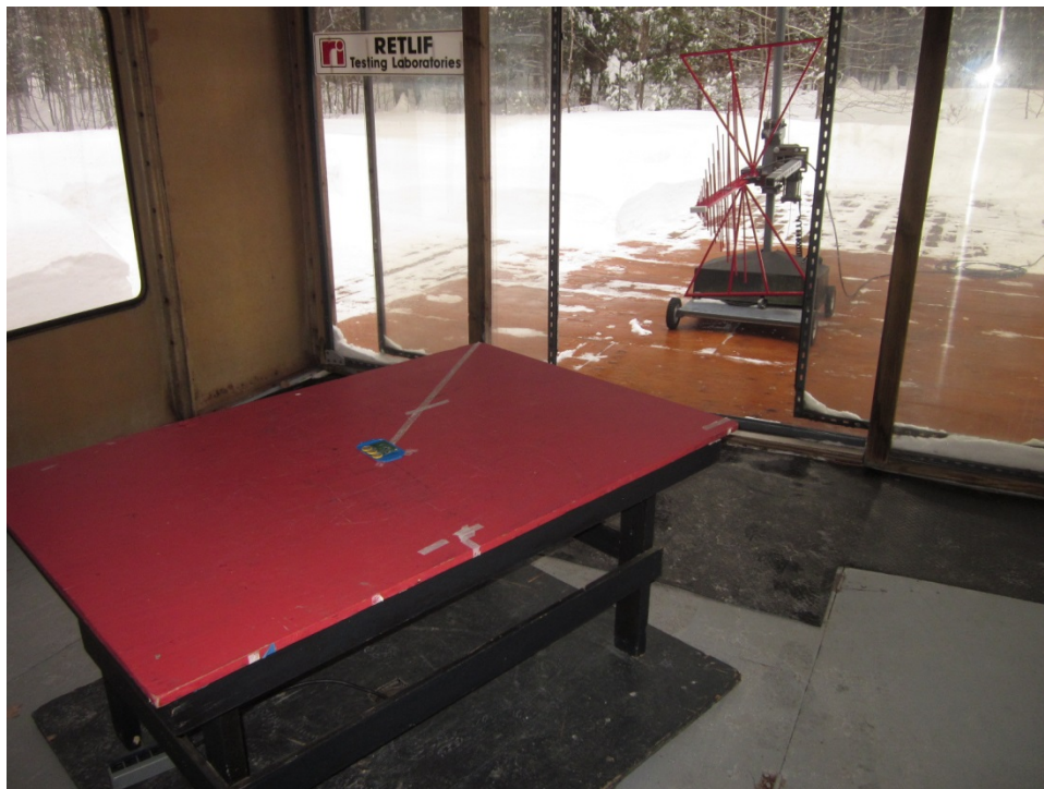
Oats Setup, 30 MHz to 1 GHz, Vertical Polarization, Model: TB-200
