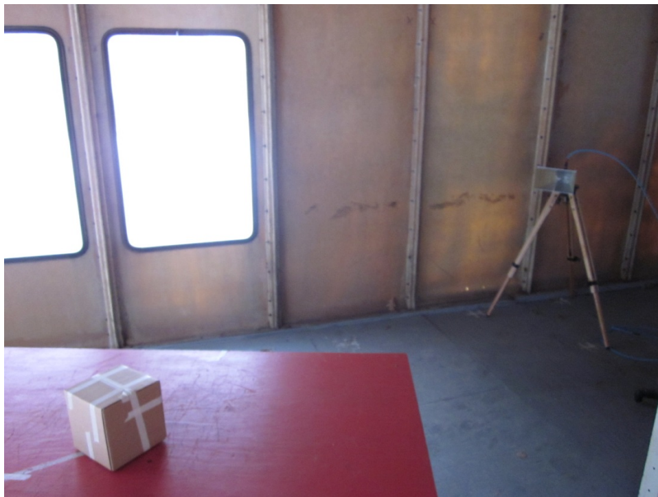
Oats Setup, 1 GHz to 18 GHz, Vertical Polarization, Model: TB-200
