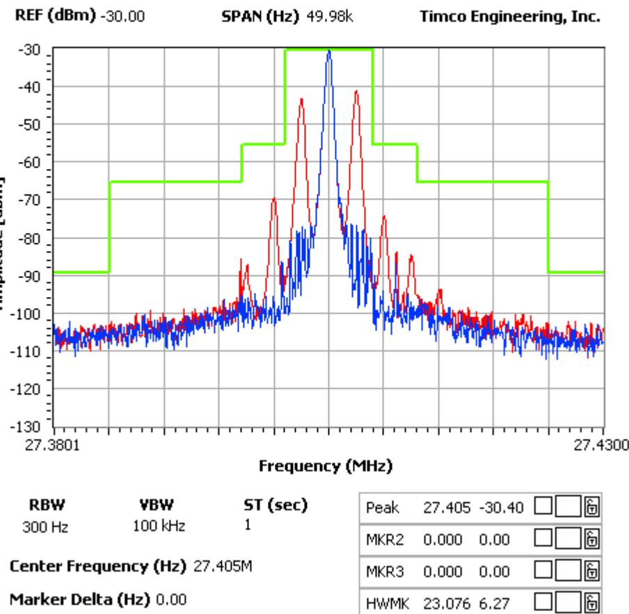
**AM mode: modulation frequency 2.5 kHz**
