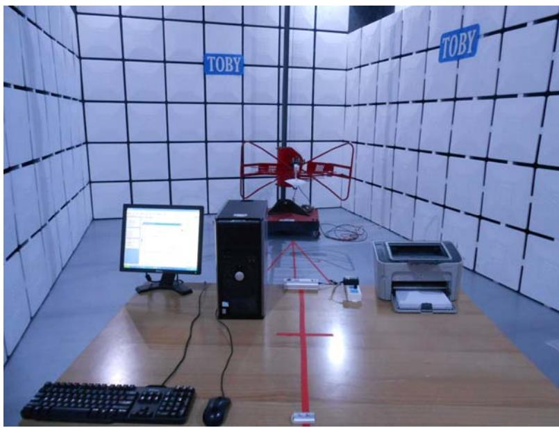
Photo of Setup for AC Mains Conducted Emission
