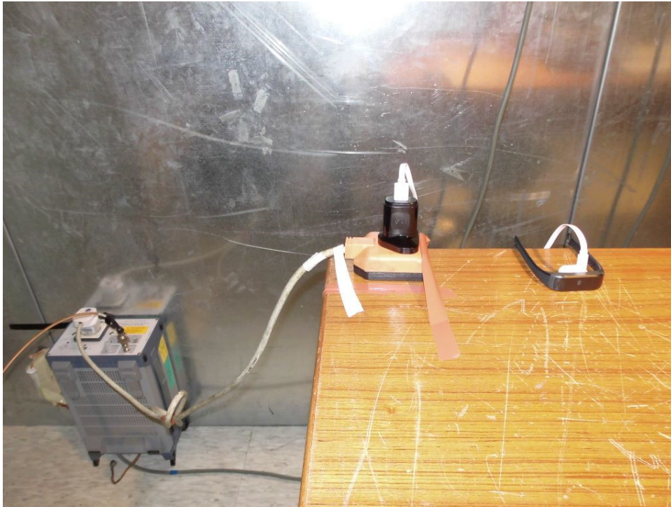
Set-up for AC mains Conducted Emission (Charging mode)
