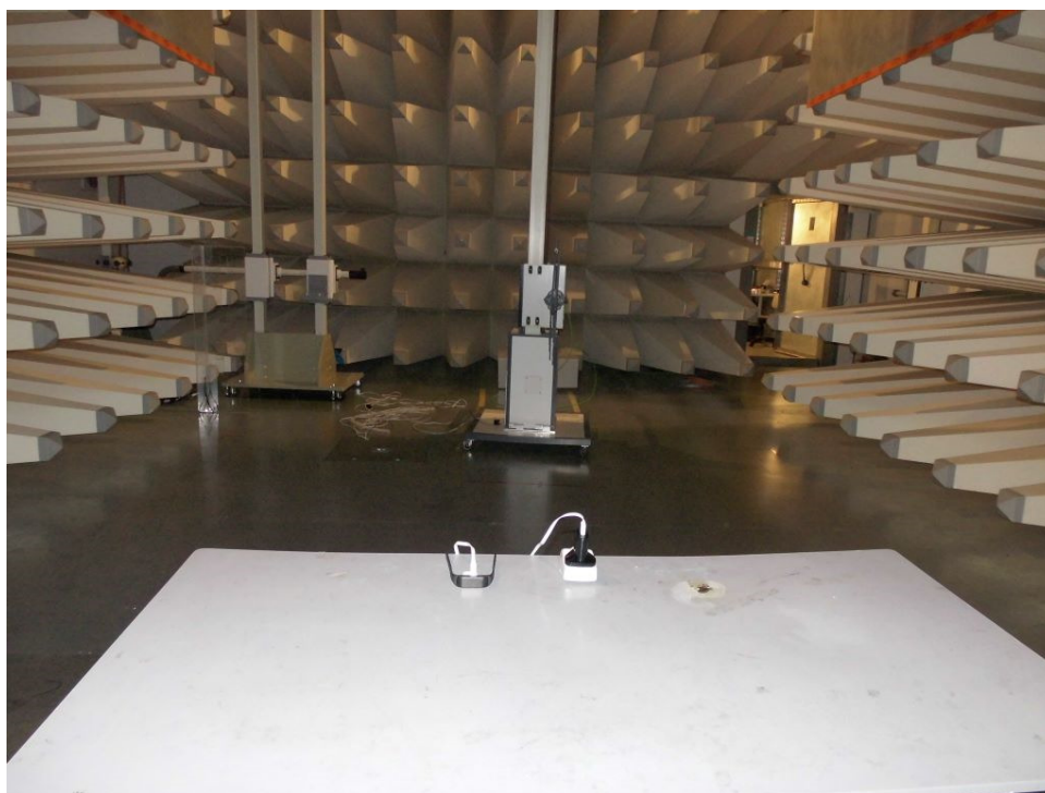
Set-up for Radiated Emission (Charging mode)
