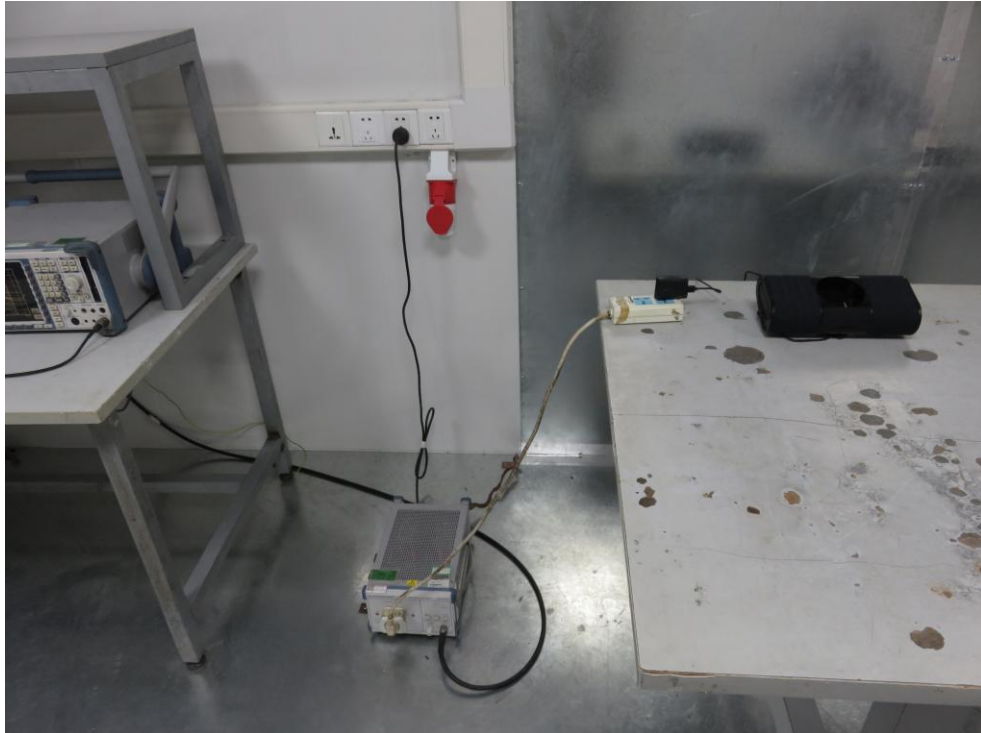
Photo of Conducted Emission Measurement
