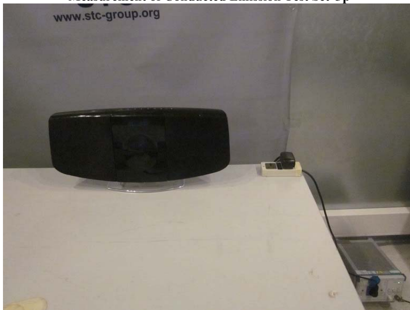
Measurement of Conducted Emission Test Set Up
