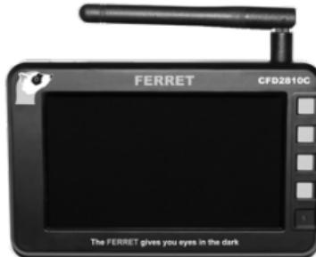
**Turn On/Off** – To turn on press the button at the top left of the display. To turn off press and hold this button for 3 seconds.
