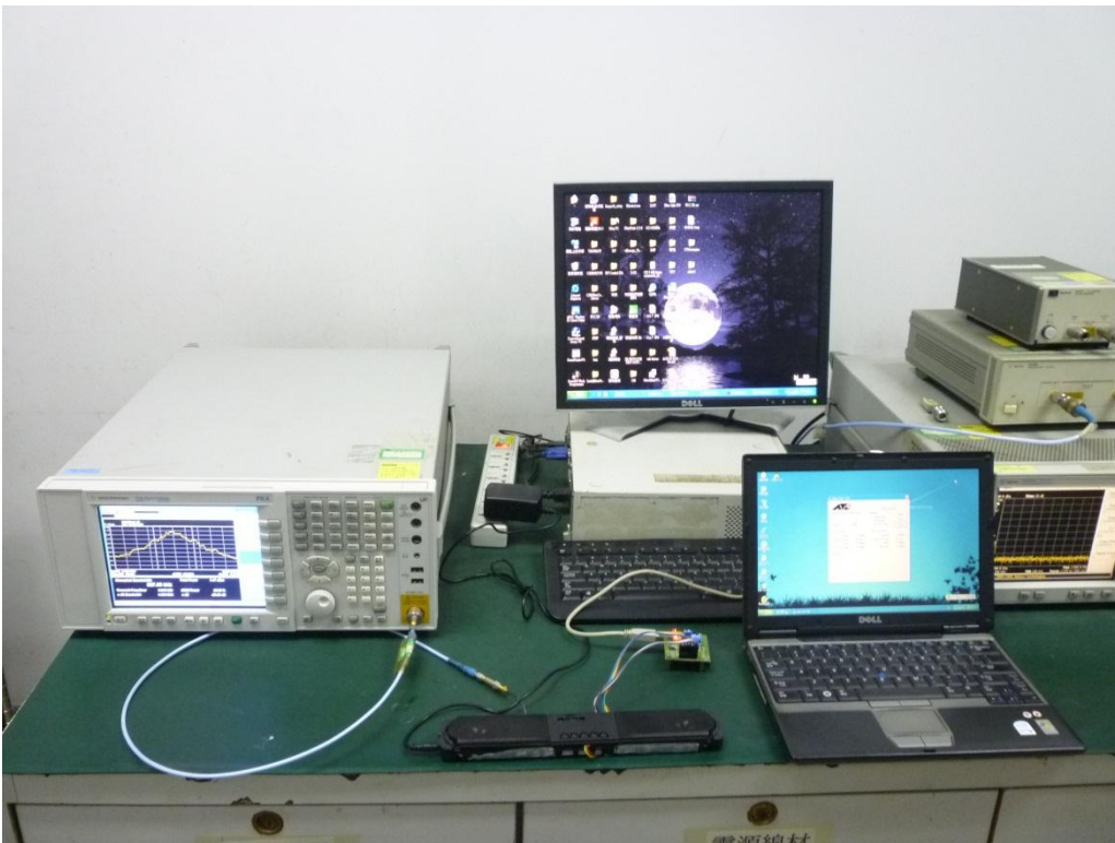
Photograph 4: Set-up for RF test
