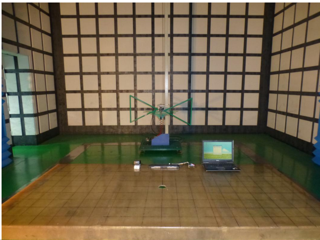
Photograph 2: Set-up for Spurious Emissions 1GHz – 18GHz
