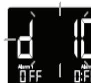
4) Next you will see the screen showing "d 01" and start flashing. Adjust the date by turning the "Rotate & Select" knob. Press the "Rotate & Select" knob to confirm the day.
