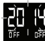
2) You can also set the clock manually by pressing and holding the "Sleep to Music" button. The screen will show "2014" and start flashing. Adjust the year by turning the "Rotate & Select" knob. Press the "Rotate & Select" knob to confirm the year.
