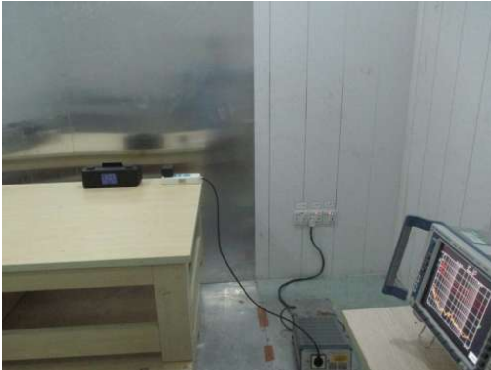
FCC RADIATED EMISSION TEST SETUP
