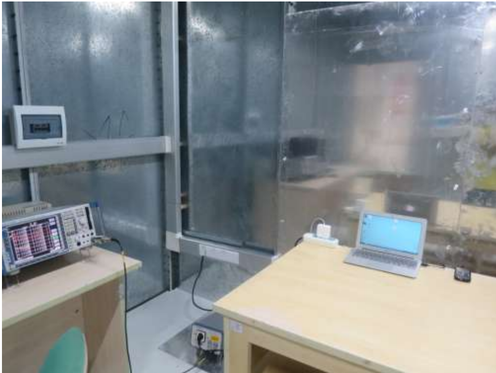
FCC RADIATED EMISSION TEST SETUP
