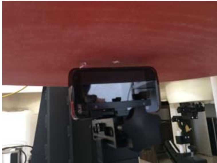
10mm Body-worn Right Side Setup Photo
