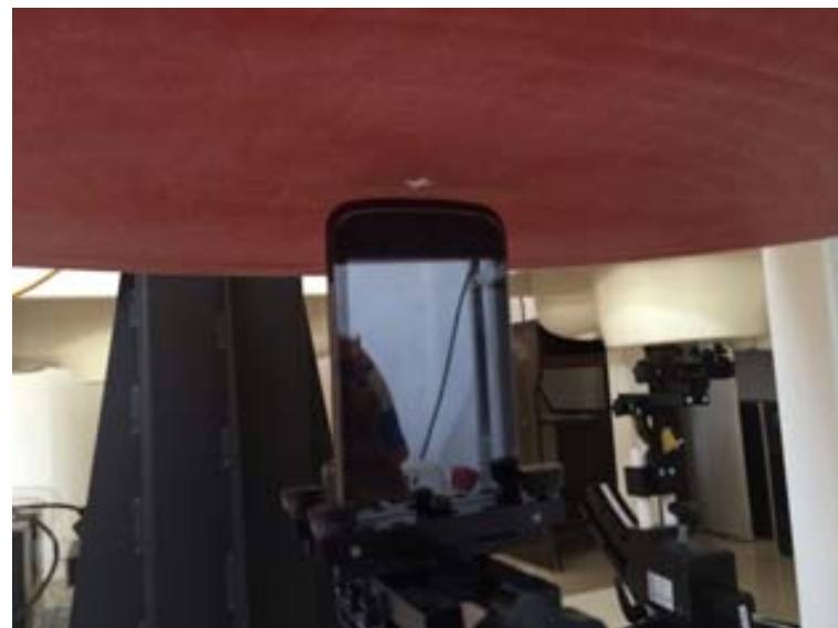
10mm Body-worn Bottom Side Setup Photo
