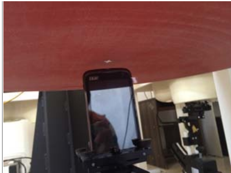
10mm Body-worn Top Side Setup Photo
