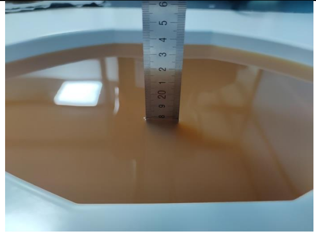
Fig. 9.2 Photo of Liquid Height for Body SAR (depth>15cm)
