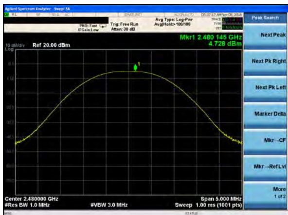
Peak output Power plot on channel 78 (1Mbps)
