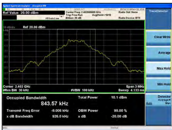
20dB Bandwidth plot on channel 39 (1Mbps)
