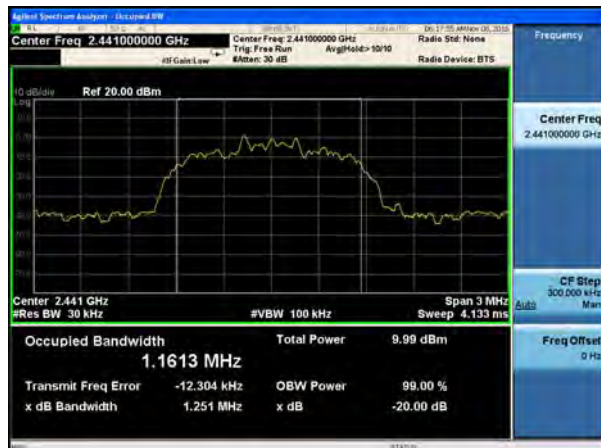
20dB Bandwidth plot on channel 78 (2Mbps)
