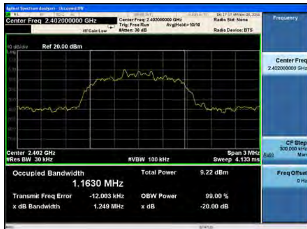
20dB Bandwidth plot on channel 39 (2Mbps)
