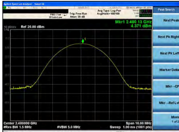
Peak output Power plot on channel 78 (2Mbps)
