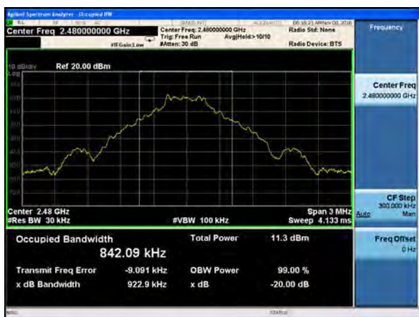
20dB Bandwidth plot on channel 78 (1Mbps)
