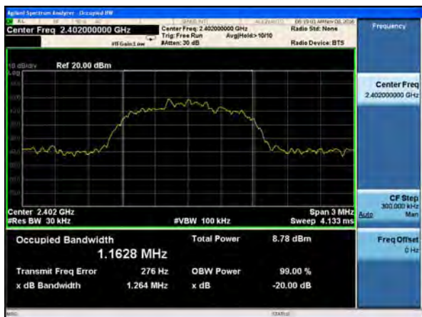
20dB Bandwidth plot on channel 39 (3Mbps)
