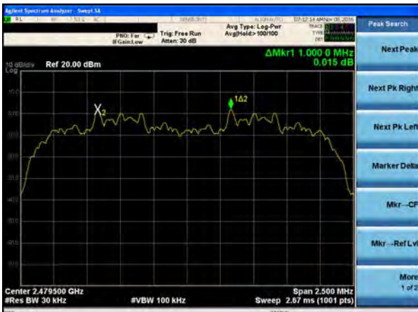
(2Mbps) Channel Separation plot on channel 77-78
