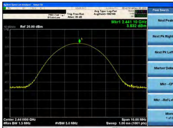
Peak output Power plot on channel 39 (2Mbps)
