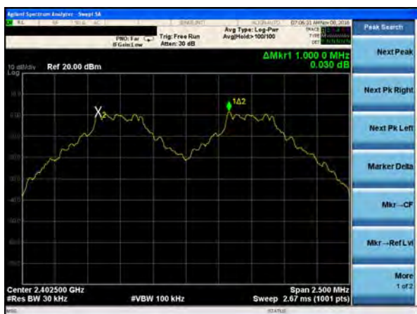
(1Mbps) Channel Separation plot on channel 39-40
