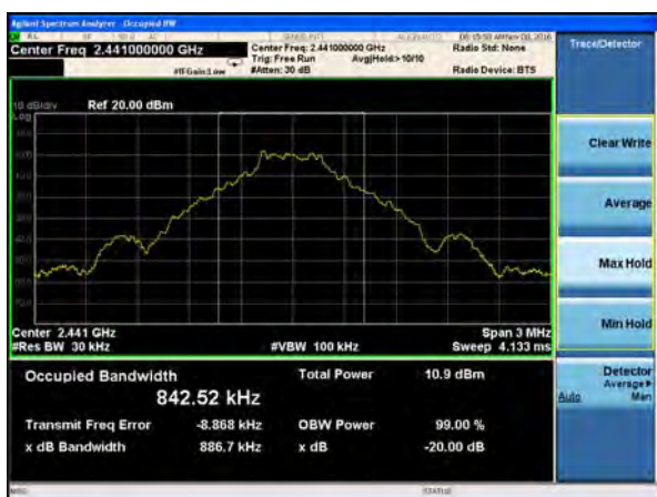
20dB Bandwidth plot on channel 78 (1Mbps)
