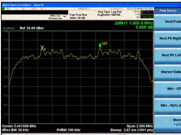
(2Mbps) Channel Separation plot on channel 39-40
