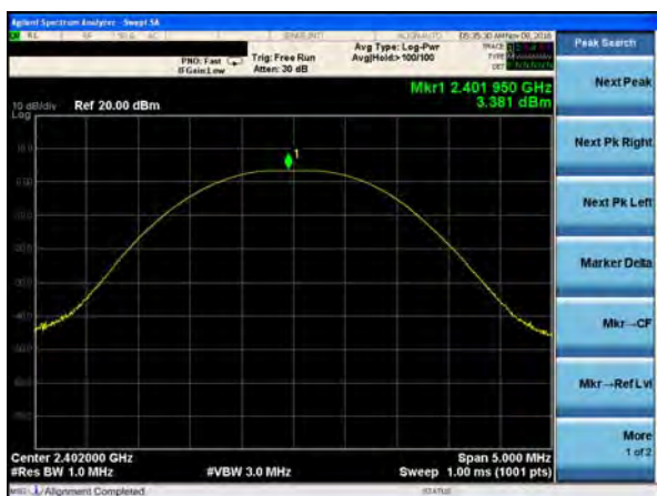
Peak output Power plot on channel 00 (1Mbps)
