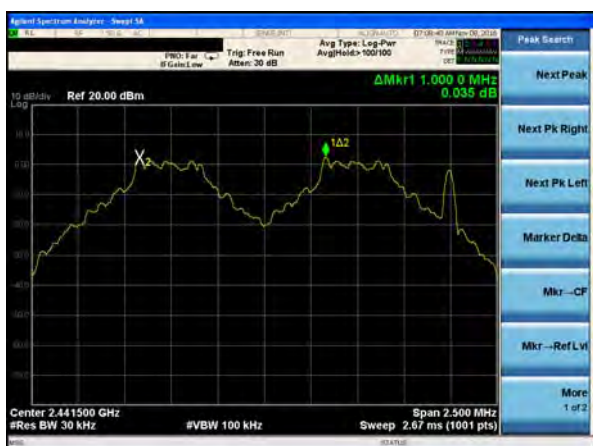
(1Mbps) Channel Separation plot on channel 39-40
