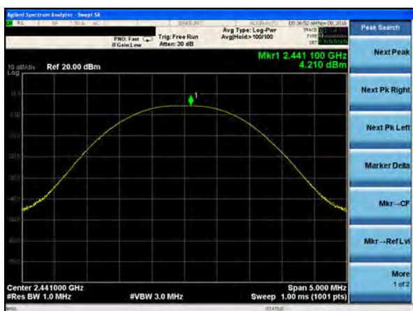
Peak output Power plot on channel 39 (1Mbps)
