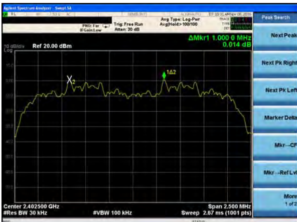
(2Mbps) Channel Separation plot on channel 39-40
