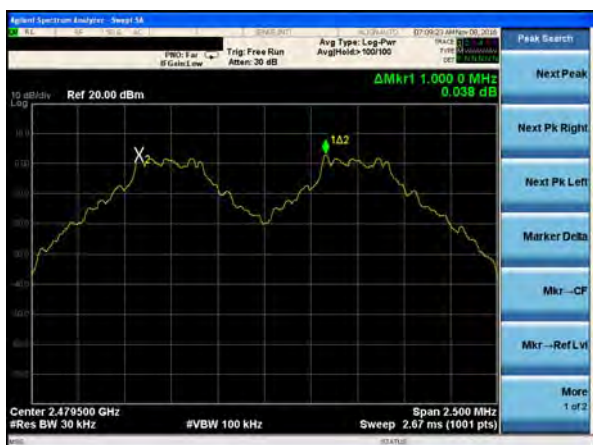
(1Mbps) Channel Separation plot on channel 77-78
