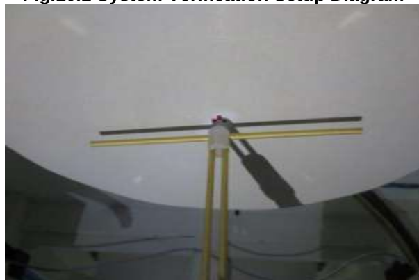
Fig.10.2 Photo of Dipole setup
