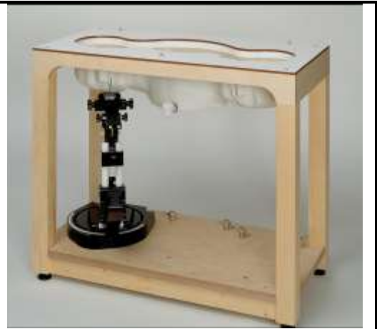
Fig. 8.7 Photo of SAM Twin Phantom
