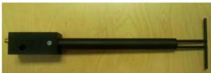
Figure 1 – MVG COMOSAR Validation Dipole
