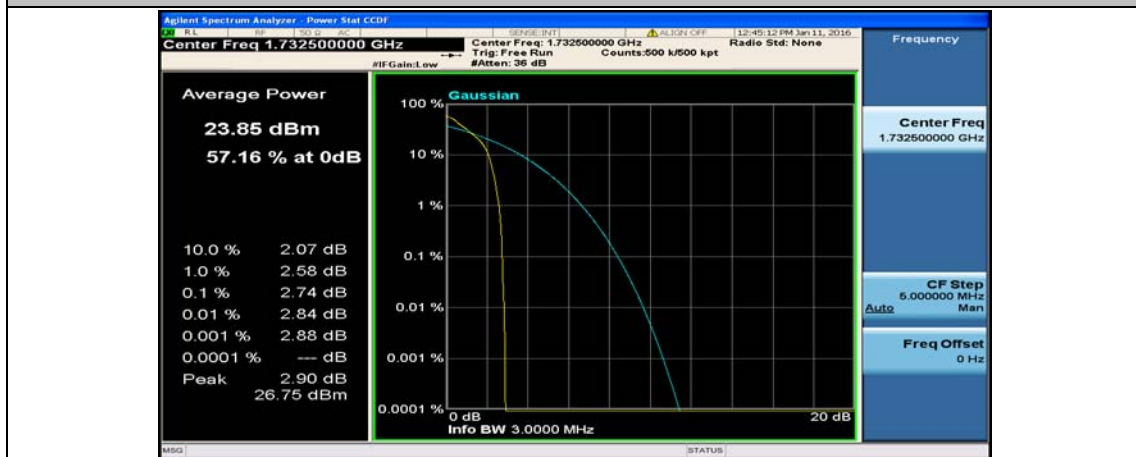
(Channel Bandwidth: 3 MHz)_MCH_QPSK_1RB#7
