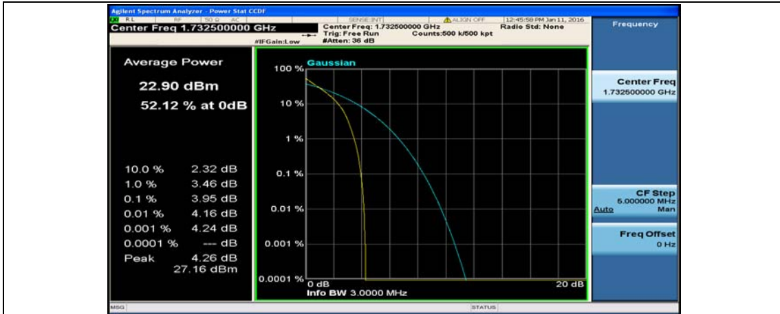
(Channel Bandwidth: 3 MHz)_MCH_QPSK_15RB#0
