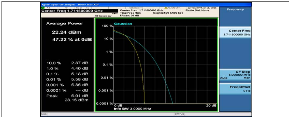
(Channel Bandwidth: 3 MHz)_MCH_16QAM_1RB#0
