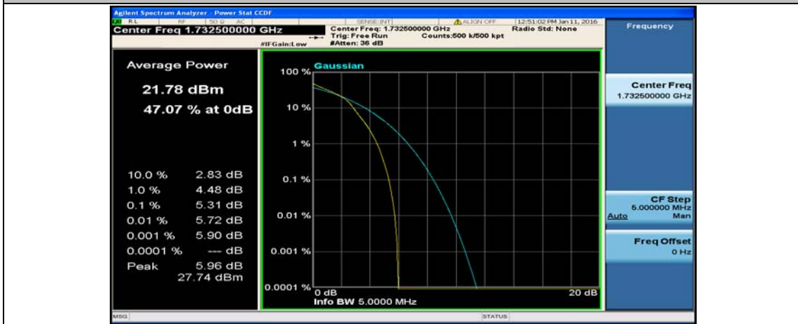
(Channel Bandwidth: 5 MHz)_MCH_16QAM_25RB#0
