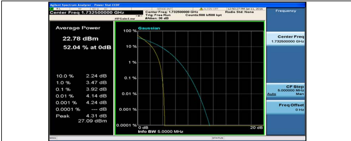
(Channel Bandwidth: 5 MHz)_MCH_QPSK_25RB#0
