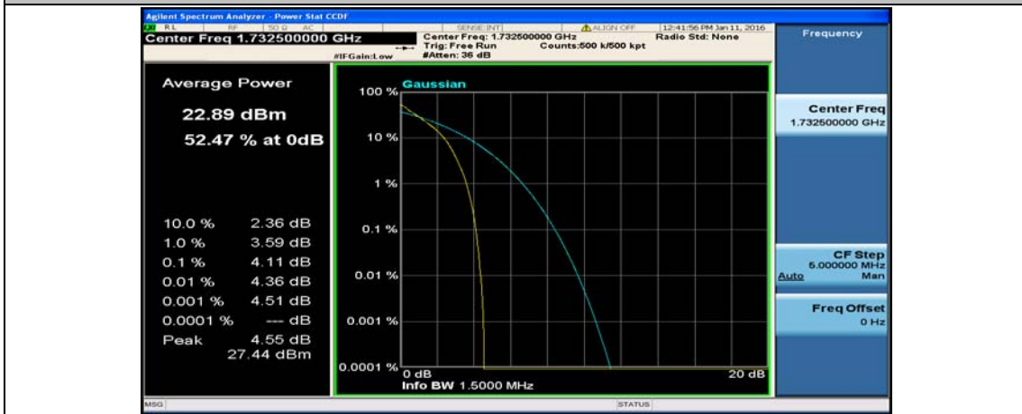
(Channel Bandwidth: 1.4 MHz)_MCH_QPSK_6RB#0
