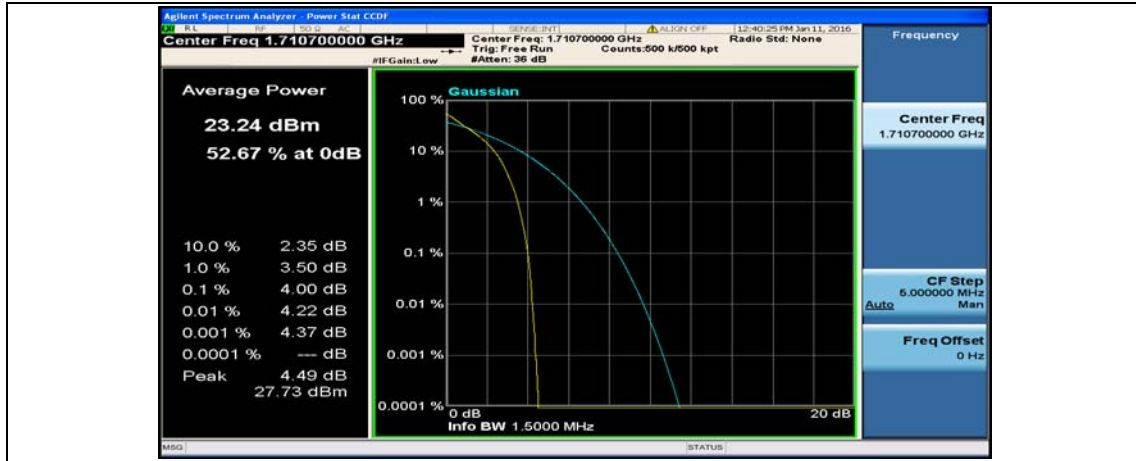
(Channel Bandwidth: 1.4 MHz)_MCH_QPSK_1RB#0
